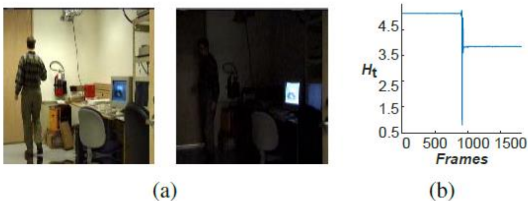
Figure 9. Example of sudden illumination change. (a) Image captures before and after the change (frame 1000) and (b) associated entropy value H_t .
