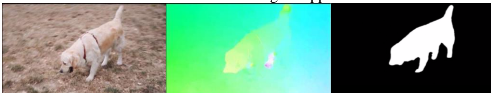
Figure 14. Example of video object segmentation. From left to right: colour image, color-coded optical flow and the improved foreground mask.
